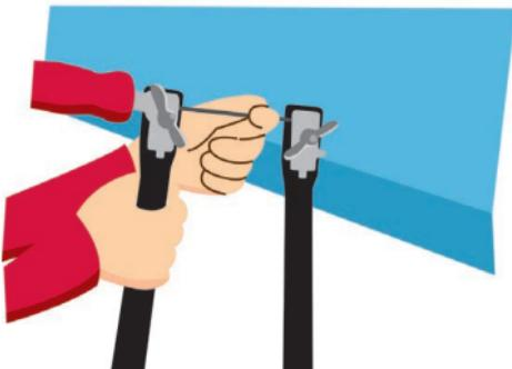
After that Siggi loosens the 2nd wing nut slightly and inserts the other end of the saw blade. That only works if he takes the handle in one hand and presses the other bow against the edge of the table to take the tension from the bow. Now he can clamp the saw blade with his free hand by placing it between the plate and the tang. Now Siggi can also tighten this wing screw with the fretsaw key.
