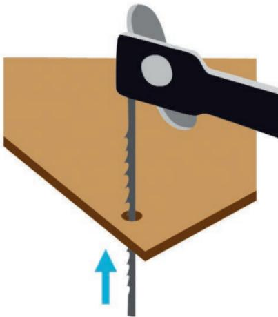
Then Sammy unclamps the saw blade on the top of the saw frame, puts it through the drilled hole and fixes it again by tightening the screw. Now Sammy can saw out the cavity. Easy, isn't it?
